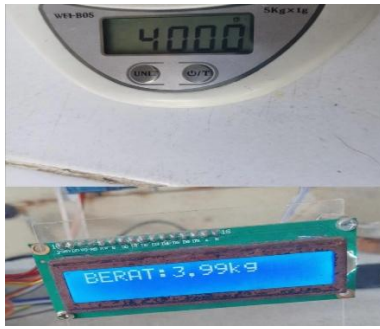
Fig. 6 Load Cell Testing 2
