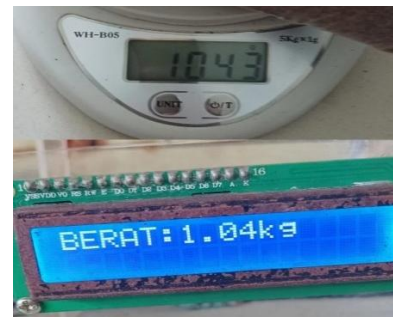
Fig. 5 Load Cell Testing 1
