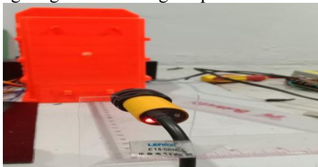
Fig. 7 E18-D80NK Proximity Sensor Testing
