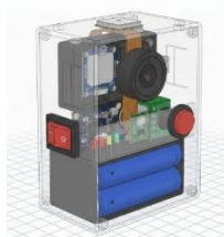
Fig. 3. Prototype design of the road damage detection hardware device.
