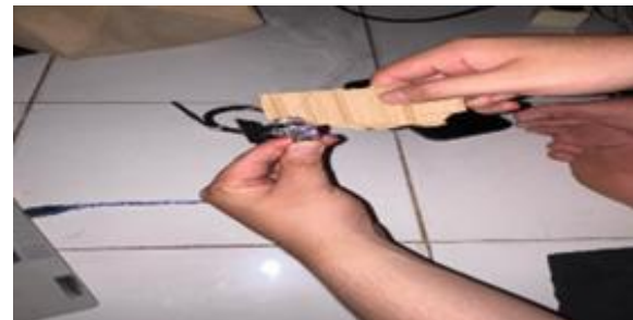
Figure 3. Testing the MQ-2 Sensor with Smoke Source
