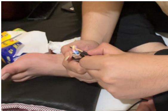
Figure 4. Testing DS18B20 Sensor with Heat Source
